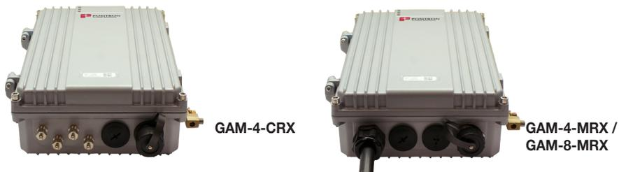
The GAM-4-MRX and GAM-8-MRX respectively have four (4) and eight (8) MIMO ports and support Reverse Power Feed (RPF) from G1001-MR devices, one per G.hn port. The GAM-4-CR has four (4) COAX ports and supports RPF mode from G1001-CR devices, one or more (in Point-to-Multipoint mode) per G.hn port.
